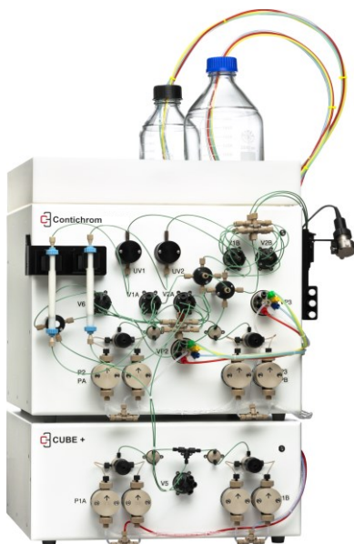
Fig. 5 Contichrom CUBE benchtop chromatography system
