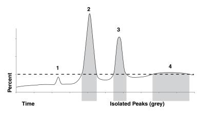
Figure 3-13 Threshold detection cuts peaks when external peak signal exceeds set percentage
