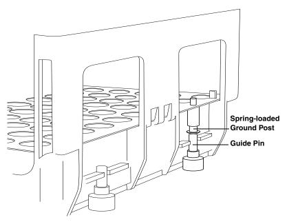
Figure 2-13 Rack installed with ground post touching guide pin
