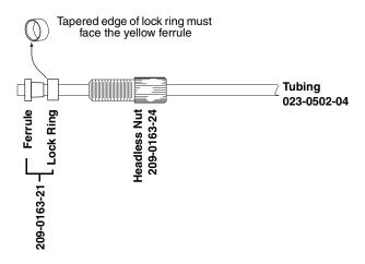
Figure 2-7 Tubing preparation
