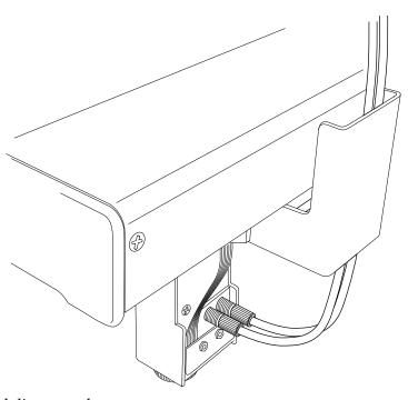
Figure 2-8 Connections to standard diverter valve
