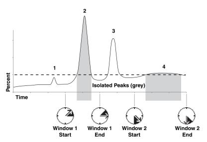
Figure 3-17 Time Windows limit the collection to specific time durations
