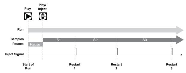
Figure 3-4 Inject options timing diagram
