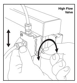
Figure 2-1 Adjusting the height of the standard (left) and high flow (right) diverter valves
