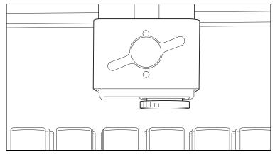
Figure 2-14 Diverter Valve adjusted with <sup>1</sup>/2 inch or 1 cm clearance (standard diverter valve shown)
