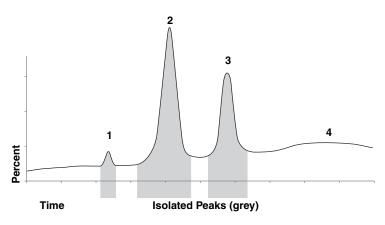
Figure 3-15 Peak Width detection cuts peaks when internal slope algorithms indicate a peak
