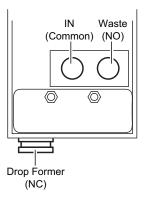
Figure 2-6 Diverter valve ports
