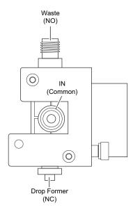
Figure 2-9 High flow diverter valve ports (front view)
